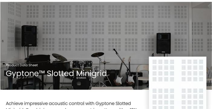
Achieve impressive acoustic control with Gyptone Slotted Minigrid. Combining a modern geometric pattern with a 13% open area, Gyptone Slotted Minigrid provides impressive levels of sound attenuation to match its good looks.
