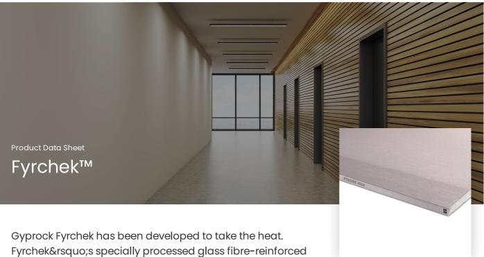
Gyprock Fyrchek has been developed to take the heat. Fyrchek's specially processed glass fibre-reinforced gypsum core makes it ideal for use in fire rated wall and ceiling systems and where improved acoustic performance is required.
