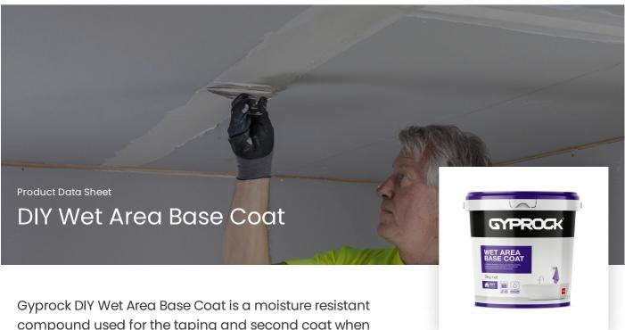
compound used for the taping and second coat when jointing plasterboard and fibre cement sheets in areas subject to moisture or high humidity.
