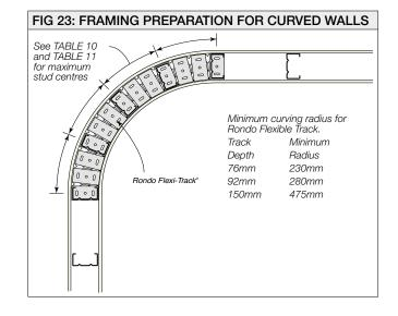
In most instances, two layers of Gyprock Flexible Plasterboard are recommended, and they can easily be flush jointed to one layer of 13mm Gyprock plasterboard for adjacent straight sections where appropriate.
