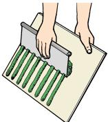
Apply Gyprock sheets with the long edges at right angles to joists or battens.
