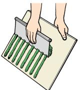
• Reinforce the butt joint with the back-blocking along the full length of the butt
