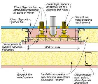
Figure 144: Plumbing Services With SilencerF - Stud Wall – Section View
