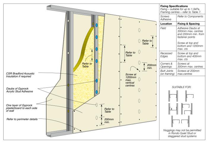
Figure 18: Non-Fire Grade Plasterboard Fixing – Vertical Sheeting – Adhesive/Fastener Fixing – Non-Tiled Areas
