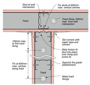
Figure 106: Wall End Detail – Plasterboard Wall To Glazing Mullion (Maintains the FRL of the wall system in which it is installed).
