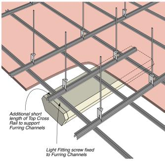
Figure 319: Surface Mounted Light Parallel To Furring Channels
