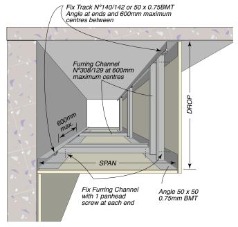
Table 36: Bulkhead Drop & Span
