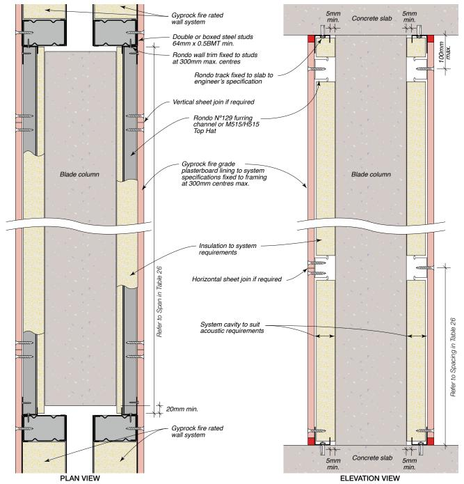
Figure 186: Discontinuous Blade Column Encasement Framing & Lining Appraisal FAR 4503.
