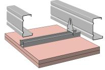
Plasterboard screw fixed to steel furring channel attached with appropriate fixing clips to masonry or steel floor/ceiling joists
