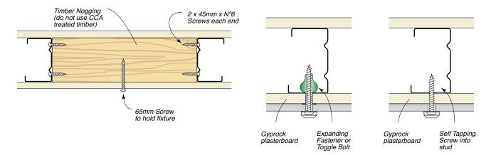
Figure 74: Heavyweight Fixtures (Eg. Wall Basins And Cisterns - Excluding Wall Hung WC Pans)
