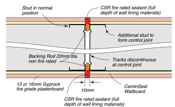
Figure 121: Control Joint For Double Layer Stud Wall Systems (Maintains the FRL of the wall system in which it is installed)
