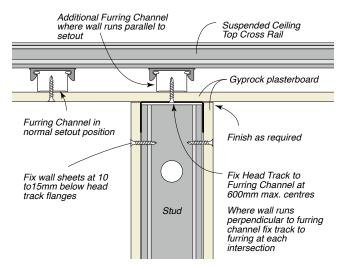
Figure 43: Head Using Aluminium Head Track
