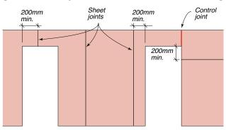
Figure 78: Joint Layout For Vertical Or Horizontal Sheeting
