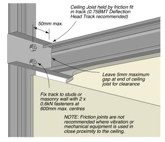
**Figure 244: Joist End Support – Mechanical Joint** Maximum Joist Span: 3.0m (single span). Maximum Joist Span: 4.0m (continuous over 2 or 3 spans).
