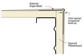
Figure 407: Procedure For Hand Jointing Of External Corners
