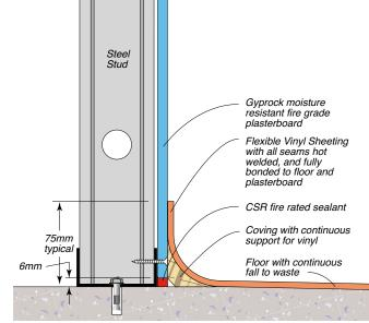
Figure 229: Perimeter Fully Bonded Vinyl Sheeting
