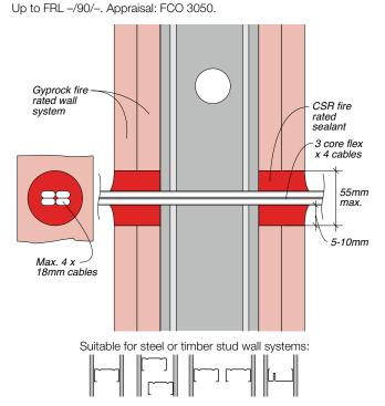
Figure 134: Cable Penetration PVC sheathed cables up to 3 cores of  $2.5mm^2$  nom. area or 7 x 0.67 metric strand
