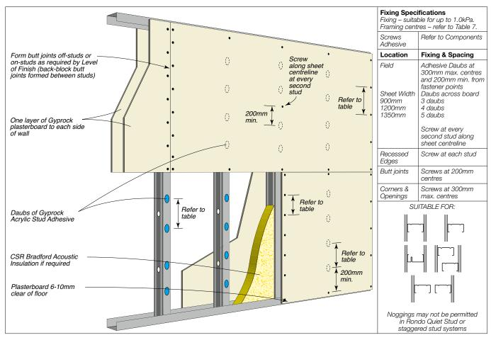
Figure 20: Non-Fire Grade Plasterboard Fixing - Horizontal Sheeting - Adhesive/Fastener Fixing - Non-Tiled Areas
