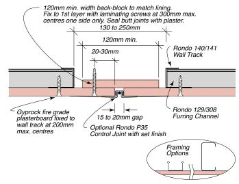
Figure 312: Control Joint Perpendicular To Steel Framing – 2 Layers – Optional Set Bead Finish (Maintains FRL and RISF of the ceiling system in which it is installed).
