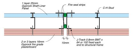
Figure 327: Typical Fire Hatch In Ceiling
