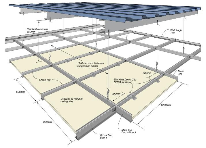
Figure 386: Typical Installation Detail - Rondo Duo Exposed Grid Suspended Ceiling System
