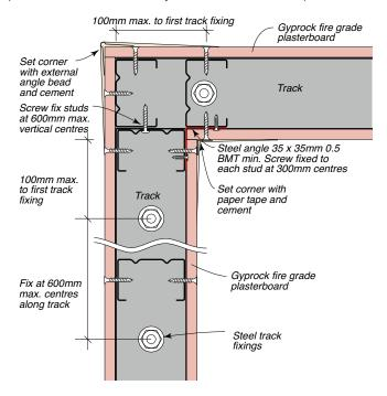
Figure 105: Junction Detail – Plasterboard To Plasterboard Walls (Maintains the FRL of the wall system in which it is installed).
