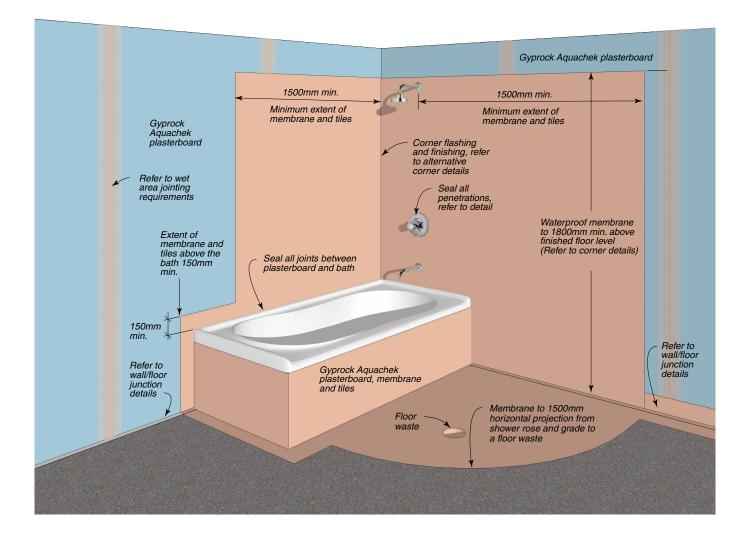
Figure 205: Membrane Detail For An Unenclosed Shower Over Bath Or Shower Area
