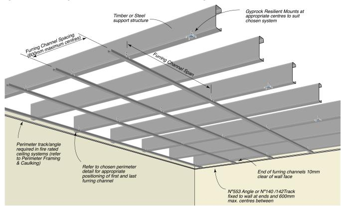
Figure 233: Steel Furring Channel Fixed With Resilient Mounts To Framing
