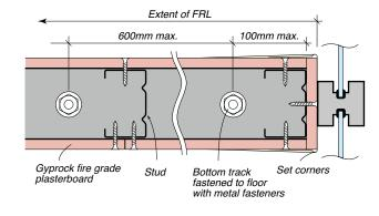
Figure 107: Junction Detail – Plasterboard To Concrete, AAC or Masonry Wall (Maintains the FRL of the wall system in which it is installed).
