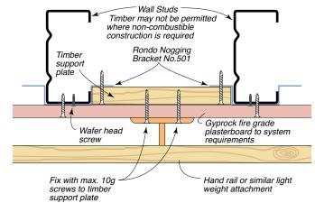
Figure 151: Typical Access Panel In Wall Appraisal: Refer to manufacturer.
