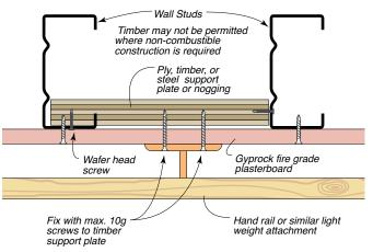
Figure 152: Light Weight Fixture Attachment – Handrails, Basins & Signs – Alternative Method Maintains the system FRL. Appraisal: FC 12946.
