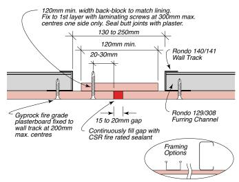
Figure 309: Control Joint Perpendicular To Steel Framing – 2 Layers – Sealant Finish
