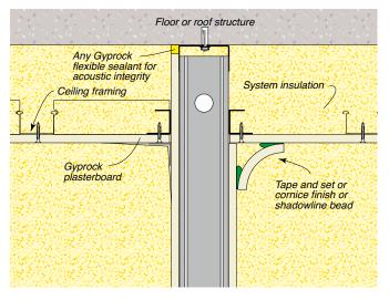
Figure 48: Wall/Ceiling Junction – Tile Lining
