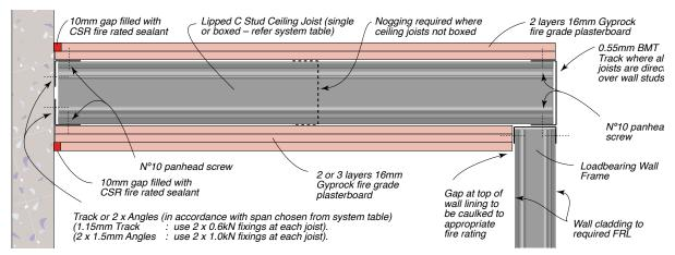
Figure 250: General Layout Of C-H Stud Ceiling Framing Lined Two Sides
