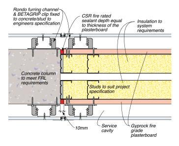
Figure 185: Blade Column To Non-Discontinuous Lightweight Wall Junction – Alternative Appraisal FC 12946
