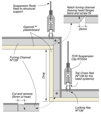
Cut through head and down legs of furring channel (leave face intact) bend and screw fix
