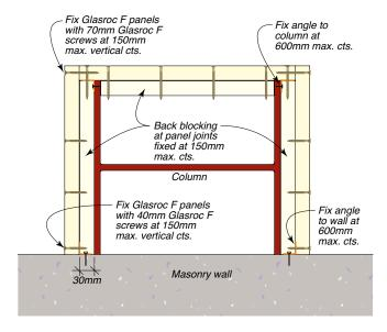
Figure 173: Three Sided Encasement Framing
