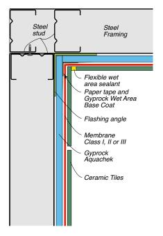
Figure 208: Internal Corner Detail – Class 2 Membrane
