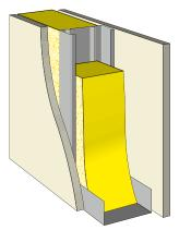
Single Stud Framing Lined One or Two Sides
