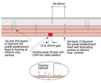
Figure 311: Control Joint Perpendicular To Steel Framing – 1 Layer – Optional Set Bead Finish
