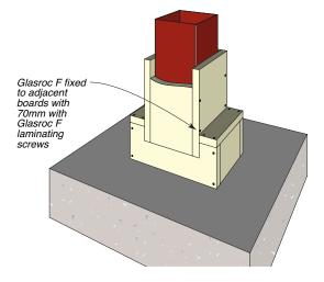
Figure 180: Flange Protection With Packers
