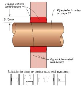
Figure 128: Pipe Penetration – Copper, Brass & Ferrous Metals
