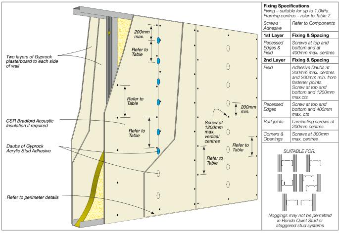
Figure 22: Non-Fire Grade Plasterboard Fixing – Two Layer – Vertical Sheeting – Adhesive/Fastener Fixing – Non-Tiled Areas
