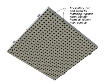
Figure 356: Joint/Screw Filling
