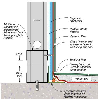
Figure 198: In situ Formed Shower Recess – Class 1 Membrane Figure 199: In situ Formed Shower Recess – Class 2 Membrane
