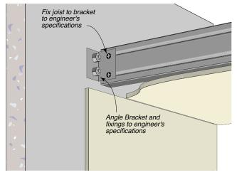
Figure 247: Joist End Support – Mechanical Joint Maximum Joist Span: 6.0m (single span).
