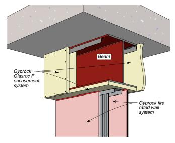
Figure 178: Three Sided Column Encasement With Wall
