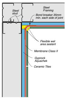
Figure 209: Internal Corner Detail – Class 3 Membrane
