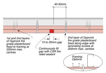
Figure 310: Control Joint Perpendicular To Steel Framing – 3 Layers – Sealant Finish
