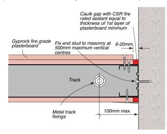
Figure 108: Junction Detail – Double Stud Wall To Single Stud Wall (Maintains the FRL of the wall system in which it is installed).
