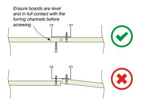
Figure 337: Rigitone Board Installation Order
