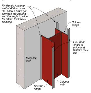
Figure 174: Three Sided Encasement Panel Fixing
