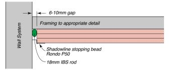
Figure 301: Suitable for 2 and 3 layer plasterboard ceiling systems.
