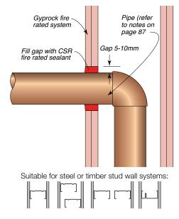
Figure 126: Pipe Penetration – Copper, Brass & Ferrous Metals Up to FRL –/120/–. Appraisal: FCO 3050.
