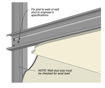
Figure 248: Bulkhead Construction For Maximum SPAN and DROP data, refer to following table.
