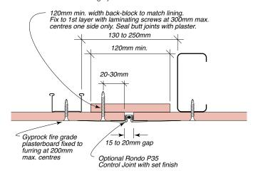
Figure 306: Control Joint Parallel To Steel Framing – 2 Layers – Expressed Joint Or Set Bead Finish (Maintains FRL and RISF of the ceiling system in which it is installed).
