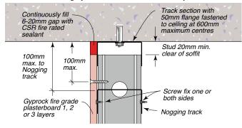
Figure 98: Head – Studs Lined One Side Only With Slotted Head Track
