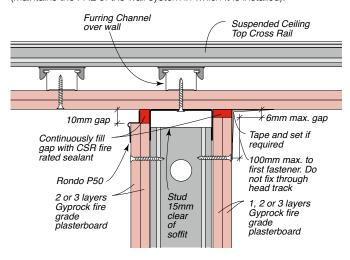
Figure 94: Wall Base Detail (Maintains the FRL of the wall system in which it is installed).
