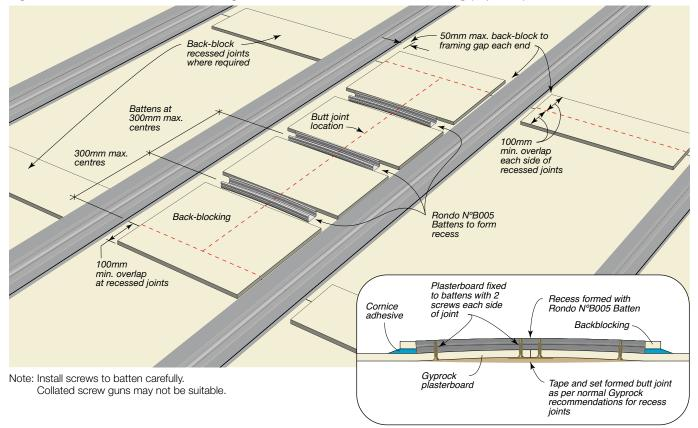
Figure 262: Butt Joint Construction Using Rondo B005 Battens And Back-Blocking (Top View)
