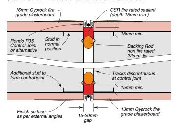
Figure 120: Control Joint For Composite Wall Systems – First Layer CeminSeal Wallboard
