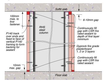
Figure 157: Fixing To Steel Hollow Section (RHS/SHS)
