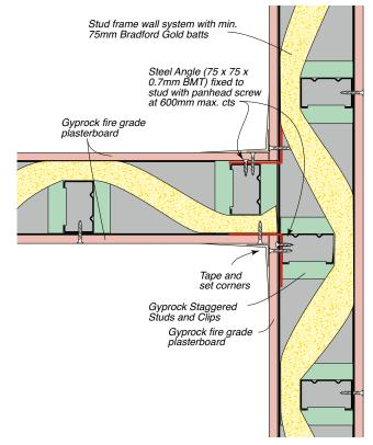
Figure 115: Junction Detail – Lost Stud Plasterboard Wall Lined Both Sides To Masonry Wall – 1, 2 Or 3 Layers Plasterboard
