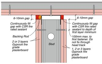
Figure 93: Wall/Ceiling Junction (Maintains the FRL of the wall system in which it is installed).
