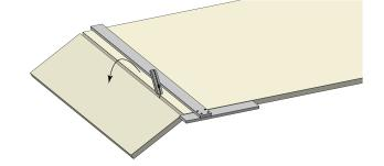
TIP: Site recessing tools are available to treat cut edges for easier jointing.
