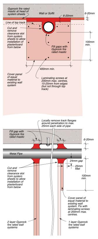
Figure 130: Penetration Detail – Metal Pipe 50 to 400mm from Wall/Soffit Junction (Up to -/120/-) Appraisal: FCO 3050.
