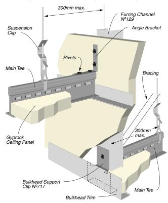
Figure 396: Suggested Bulkhead Detail (Maximum Drop 600mm) Horizontal Exposed Grid/Vertical Screw-Up System
