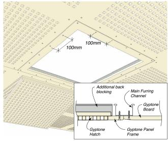
Set the joint between the board and the Access Panel frame using the Gyprock three coat jointing system, sanding smooth between coats, and omitting the application of Paper Tape (this is not required).
