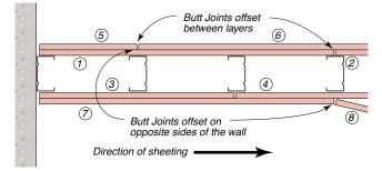
Joints are not to coincide with the edge of openings (eg doorways or windows). Sheets are to be laid so that any joint falls a minimum of 200mm from the edge of an opening. Avoid butt joints over single doorways and cavity sliding doors wherever possible. Refer to the following detail.
