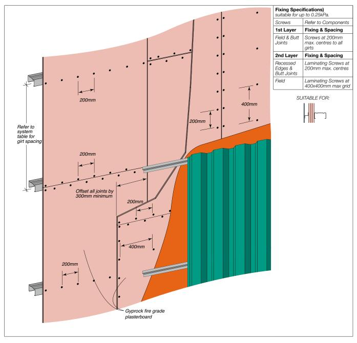
Figure 89: Fire Fire Grade Plasterboard To Steel Frame External Wall System Two Or Three Layer – Vertical Sheeting – Screw Fixing
