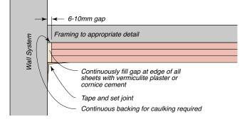
Figure 298: Suitable for 1, 2 and 3 layer plasterboard ceiling systems.
