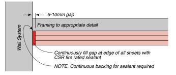
Figure 297: Suitable for 1, 2 and 3 layer plasterboard ceiling systems.
