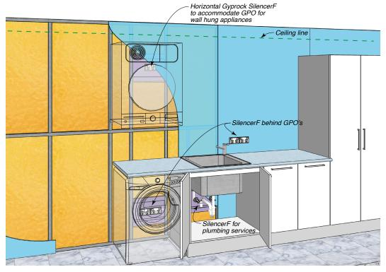
Figure 146: Typical Applications For Gyprock SilencerF – Laundry
