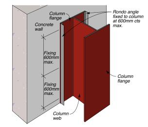
Figure 169: Three Sided Encasement Framing
