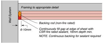
Figure 294: Suitable for 2 and 3 layer plasterboard ceiling systems.
