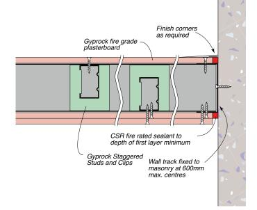
Figure 114: Wall/Wall Junction – Staggered Studs (Maintains the FRL of the wall system in which it is installed).
