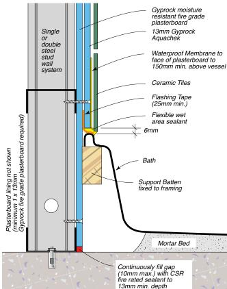
Figure 221: In situ Formed Shower Recess Ceramic Tiled – Double Layer Gyprock Moisture Resistant Fire Grade Plasterboard
