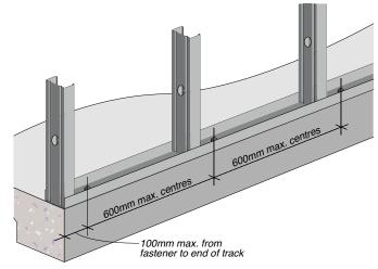
Figure 96: Head/Base – Studs Lined One Side Only With Additional Nogging Near Top Of Wall (Maintains the FRL of the wall system in which it is installed).
