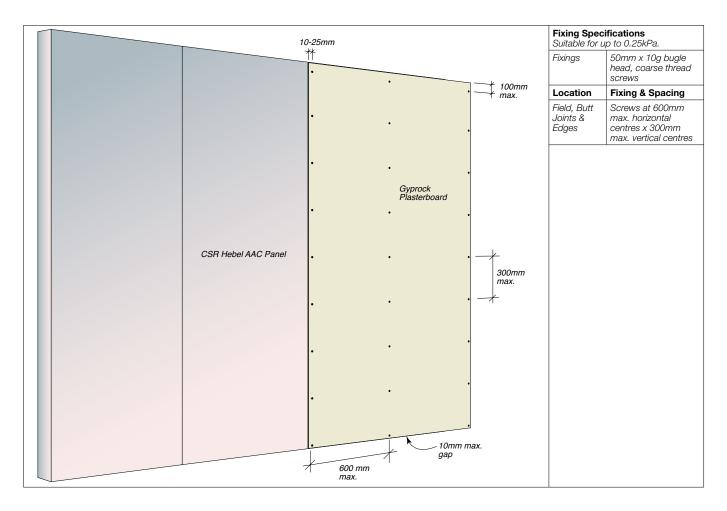
Figure 28: Non-Fire Grade Plasterboard Fixing To Hebel AAC Wall - Vertical Sheeting - Screw Fixing - Non-Tiled Areas
