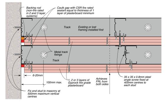
Figure 116: Junction Detail – Lost Stud Plasterboard Wall Lined One Side To Masonry Wall – 1, 2 Or 3 Layers Plasterboard
