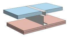
Plasterboard screw fixed under C-H studs with Gyprock Shaft Liner Panel fitted to framing above
