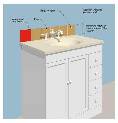
Figure 213: Typical Hand Basin – Membrane/Tiling Detail
