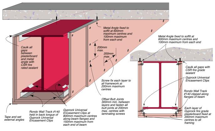
Figure 162: Steel Beam Encasement System - Fire Rated - Three Sided Plasterboard Fixing
