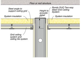
Figure 49: Wall/Ceiling Junction - Tile Lining
