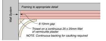
Figure 296: Suitable for 1, 2 and 3 layer plasterboard ceiling systems.
