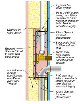
Figure 145: Plumbing Services With SilencerF - Stud Wall – Plan View
