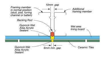
**Figure 56: Vertical Control Joint – Steel Stud Wall System** (Maintains acoustic integrity of the wall system in which it is installed). For R<sub>W</sub> up to 40, use backing rod only detail. For R<sub>W</sub> greater than 40, use backing rod and sealant detail.
