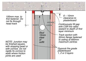
Figure 91: Deflection Head (Maintains the FRL of the wall system in which it is installed).
