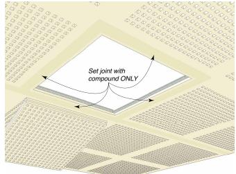
All edges of both the frame and the hatch should be painted twice to reinforce them before the hatch is placed in position.
