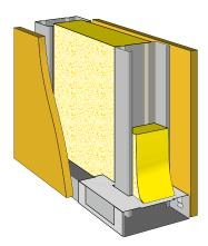
Staggered Stud Framing Lined Two Sides
