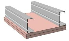
Plasterboard adhesive and/or fastener fixed directly to steel floor/ ceiling joists
