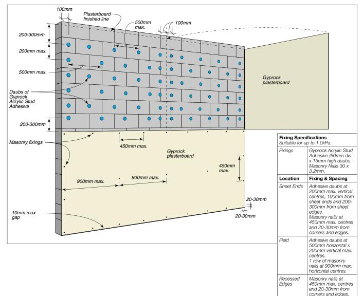
Figure 32: Plasterboard Fixing To Masonry – Horizontal Sheeting – Fastener & Gyprock Acrylic Stud Adhesive Fixing – Non-Tiled Areas
