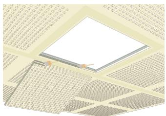
Note: When removing the hatch, ensure it is placed with the reverse side in contact with the wall or supporting surface. Avoid contact with the finished face.
