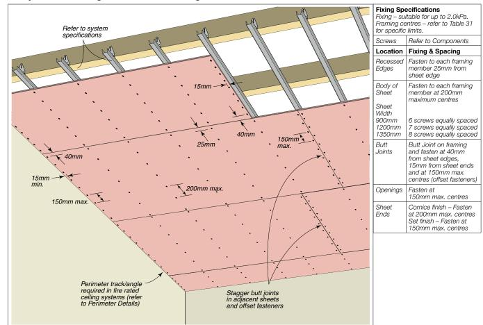
Figure 278: Fire Grade Plasterboard Fixing – Single Layer – Screw Fixing – For Systems With Lining Above Or Below Framing
