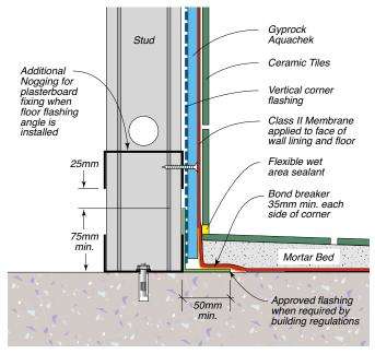
Figure 200: In situ Formed Shower Recess – Class 3 Membrane
