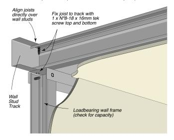
**Figure 245: Joist End Support – Mechanical Joint** Maximum Joist Span: 3.0m (single span). Maximum Joist Span: 4.0m (continuous over 2 or 3 spans).
