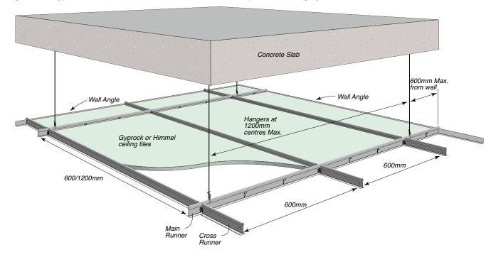
Figure 384: Typical Installation Detail – Himmel Steel Grid Suspended Ceiling System
