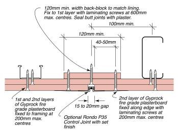
Figure 307: Control Joint Parallel To Steel Framing – 3 Layers – Expressed Joint Or Set Bead Finish Maintains FRL of the ceiling system in which it is installed.
