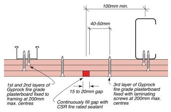
Figure 305: Control Joint Parallel To Steel Framing – 1 Layer – Expressed Joint Or Set Bead Finish Maintains FRL of the ceiling system in which it is installed.
