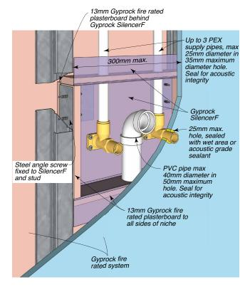
Figure 142: Plumbing Services Niche - Double Stud Wall – Section View
