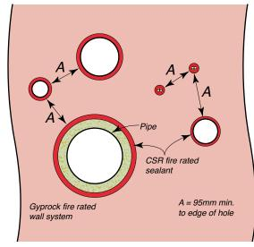
Figure 124: Pipe Penetration – Copper, Brass & Ferrous Metals Up to FRL –/90/–. Appraisal: FCO 3050.
