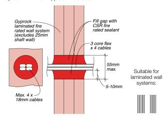
Figure 135: Cable Penetration
