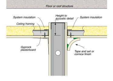
Figure 276: Wall/Ceiling Junction - Plasterboard Lining
