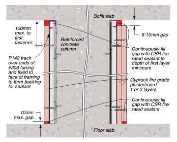
Figure 165: Plasterboard Fixed To Steel Furring
