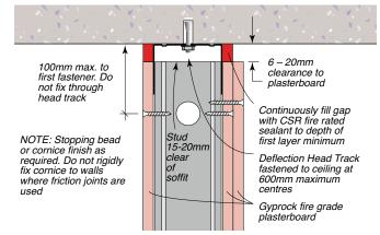
Figure 92: Wall/Ceiling Junction (Maintains the FRL of the wall system in which it is installed).
