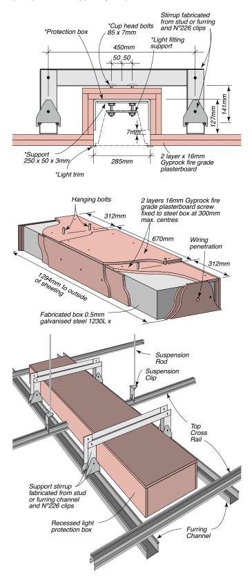
Figure 318: Surface Mounted Light Perpendicular To Furring Channels
