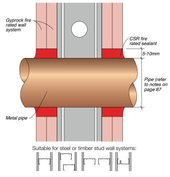
**Figure 127: Pipe Penetration – Copper, Brass & Ferrous Metals** Up to FRL –/90/–. Appraisal: FCO 3050.
