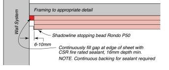
Figure 295: Suitable for 1, 2 and 3 layer plasterboard ceiling systems.
