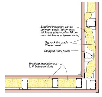
Figure 113: Wall/Wall Junction – Staggered Stud Wall To Masonry Wall
