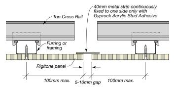
NOTE: To maintain appearance, ensure Gyprock Acrylic Stud Adhesive does not intrude into the gap.
