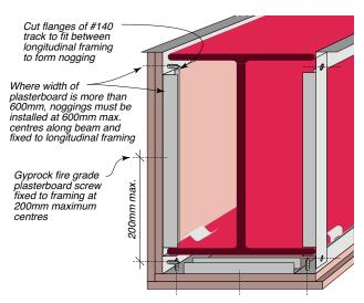
Figure 160: Beam/Wall Junction Detail
