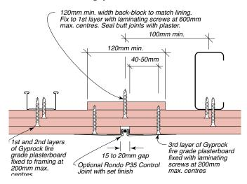
Figure 308: Control Joint Perpendicular To Steel Framing – 1 Layer – Sealant Finish
