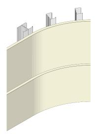
Curved Stud Framing Lined One or Two Sides
