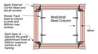
Figure 158: Plasterboard Fixing To Steel Universal Section Column
