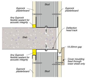
Figure 60: Horizontal Control Joint – With P35 Control Joint
