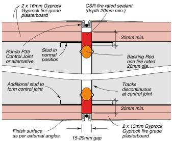
Figure 122: Control Joint For Masonry Wall – Plasterboard On Furring Channel
