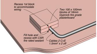
Figure 317: Recessed Light Box In Suspended Steel Frame Ceiling
