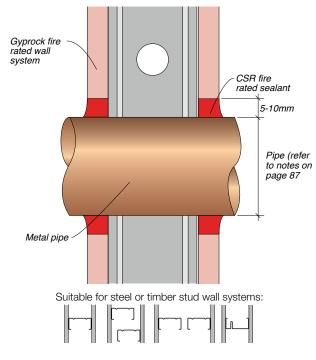
Figure 129: Penetration Detail – Metal Pipe 6 to 20mm from Wall/Soffit Junction (Up to -/120/-) Appraisal: FCO 3050.
