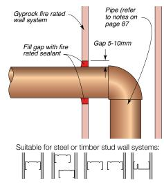
Figure 125: Pipe Penetration – Copper, Brass & Ferrous Metals Up to FRL –/120/–. Appraisal: FCO 3050.
