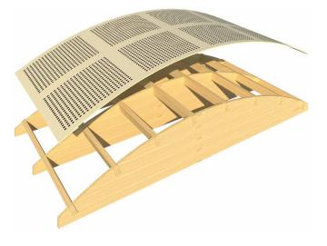
Figure 371: Curving Flexible Board Over Template
