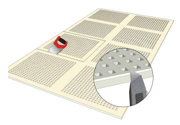
Install the Gyptone sheet onto the ceiling frame. Additional back blocking must be installed on the two unsupported hatch edges; use an offcut of furring channel cut 10mm short of the main channels. Screw fix panel to framing at 100mm centres.
