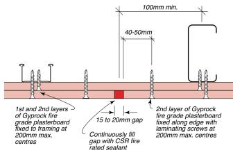
Figure 304: Control Joint Parallel To Steel Framing – 3 Layers – Sealant Finish
