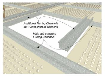
Screw fix the Access Panel frame to the furring channels on all four sides, ensure screw placement is at 100mm centres. This must be completed on all four edges to ensure all joints are stable and to avoid reflective cracking.
