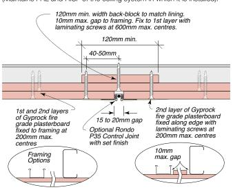
Figure 313: Control Joint Perpendicular To Steel Framing – 3 Layers – Optional Set Bead Finish
