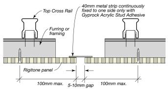
NOTE: To maintain appearance, ensure Gyprock Acrylic Stud Adhesive does not intrude into the gap.
