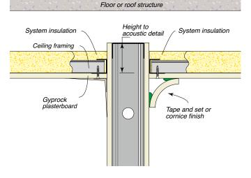
Figure 46: Wall/Ceiling Junction – Plasterboard Lining
