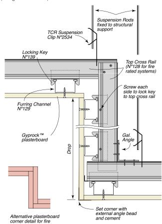
Figure 238: Suspended Bulkheads
