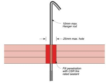
**Figure 323: Hanging Rod Through 1 Layer Ceiling** (Maintains FRL and RISF of the ceiling system were applicable.) Appraisal: EWFA 28014.
