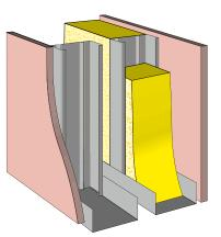
Double Stud Framing Lined Two Sides
